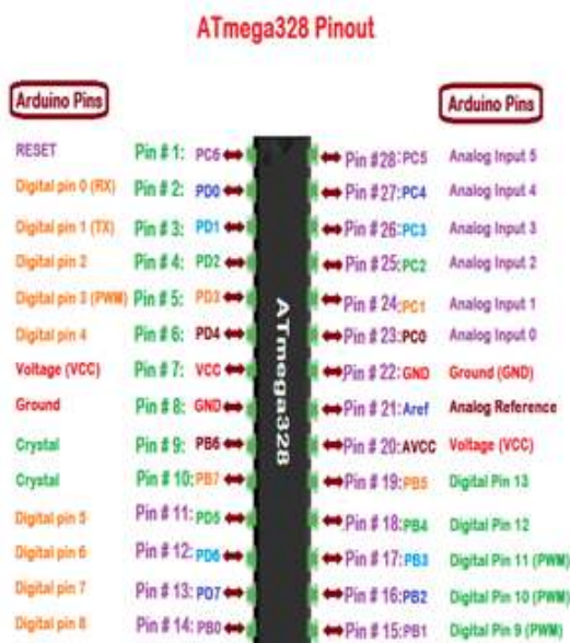
Fig-2. Pin description of ATmega328 microcontroller
